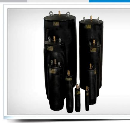
These plugs are molded of special NR-SRB rubber, reinforced with Kevlar tire cording. The working pressure of all plugs is tested three times to ensure durability and safety. Due to their light weight and short length, pipe plugs are easy to handle even in large diameter sizes. Available in multi-size versions for pipes from 35 to 1200mm in diameter. All plugs are equipped with quick-connect couplings and nipples. Reinforcement sleeves are available for heavy duty use.
